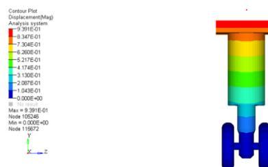
First mode shape of Landing gear system.
