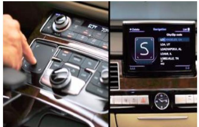
The best aspect about MMI contact is that it enables drivers to input characters just with the aid of the use of a finger to “write” at the exact touchpad. This has a huge range of packages including keying in addresses for navigation functions, coming into smartphone numbers or sincerely selecting songs to play. MMI contact also has aid for a number of languages besides English.
