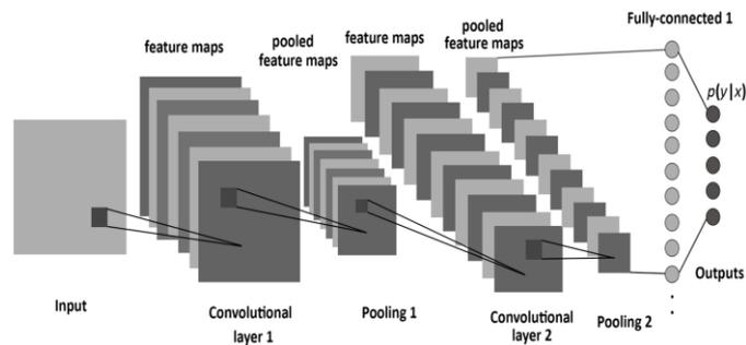
Figure 1: CNN Architecture
