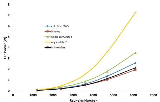
Fig -9: Fan power Vs Reynolds number plot.
