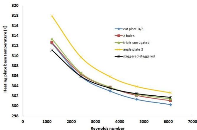
Fig -7: Variation of heating plate base temperature with Reynolds number
