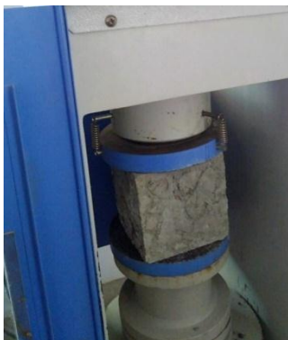
Fig -1: Compressive strength test
