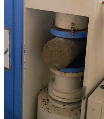
Fig -2: Split tensile strength test
