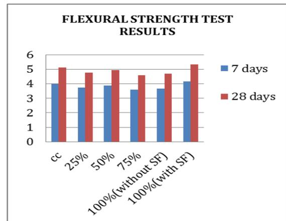
**Fig-6:** comparisons of flexural strength
