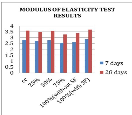
**Fig-5:** comparison of modulus of elasticity test
