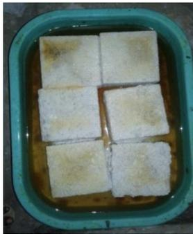
Fig-7: Acid attack test
