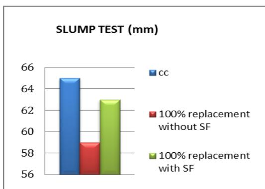
**Fig.2:**slump test results
