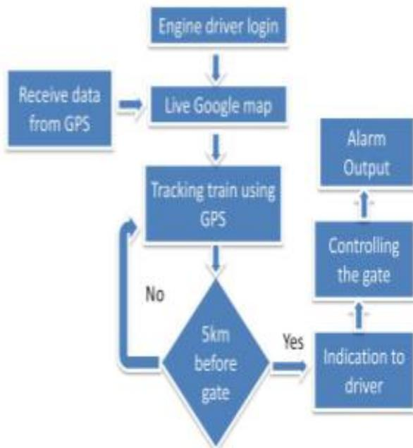
Figure 2.12: System using GPS and GSM [8]
