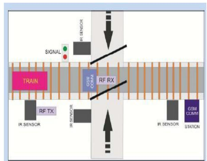
Figure 1.3: Automated Railway Crossing System [10]
