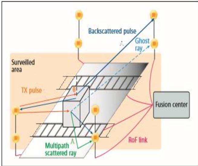
Figure 2.9: Architecture of the level crossing surveillance system with the FOS UWB radar. [4]
