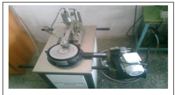
Fig.1- Top View of Pin-On-Disc Machine
