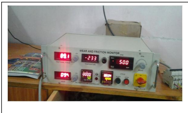
Fig.2- Wear and Friction Monitor
