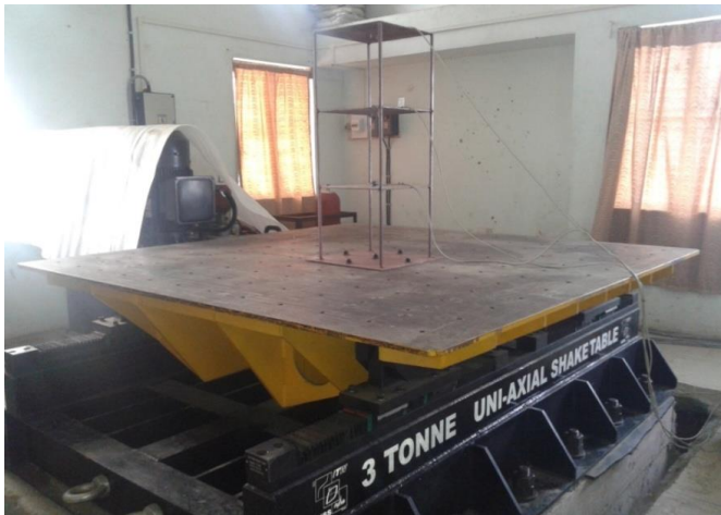
Fig -2: Model fixed on Shake Table
