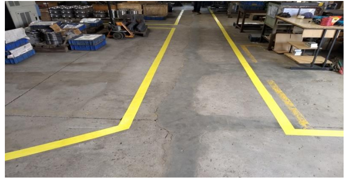
Figure 10 Change in Gangway and Plant Layout in the final stage (Observing More Space Available for Material in the Left Side of the Image)
