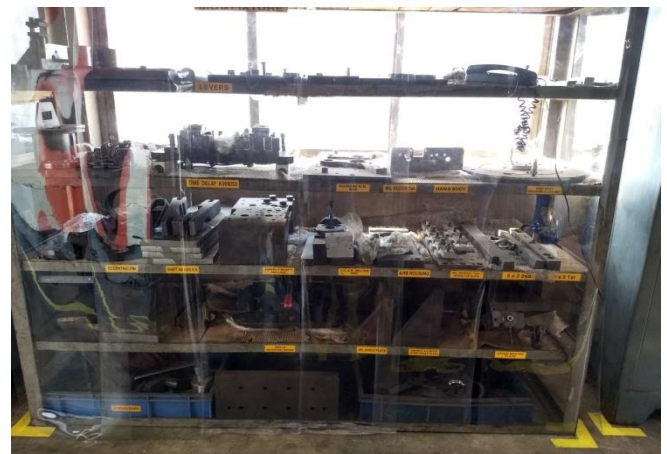
Figure 6 After image of the rack (Racks are covered by Curtains Made up of Rexist Material for Protection from Dirt)
