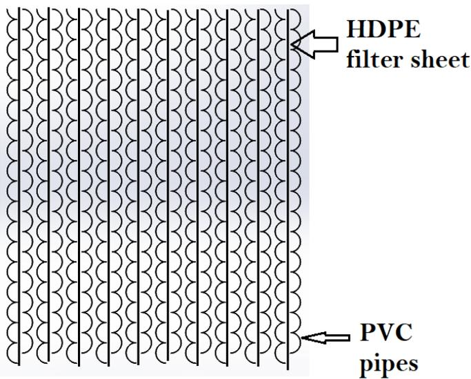
Figure 4: Carbon Dioxide filter (Top View)
