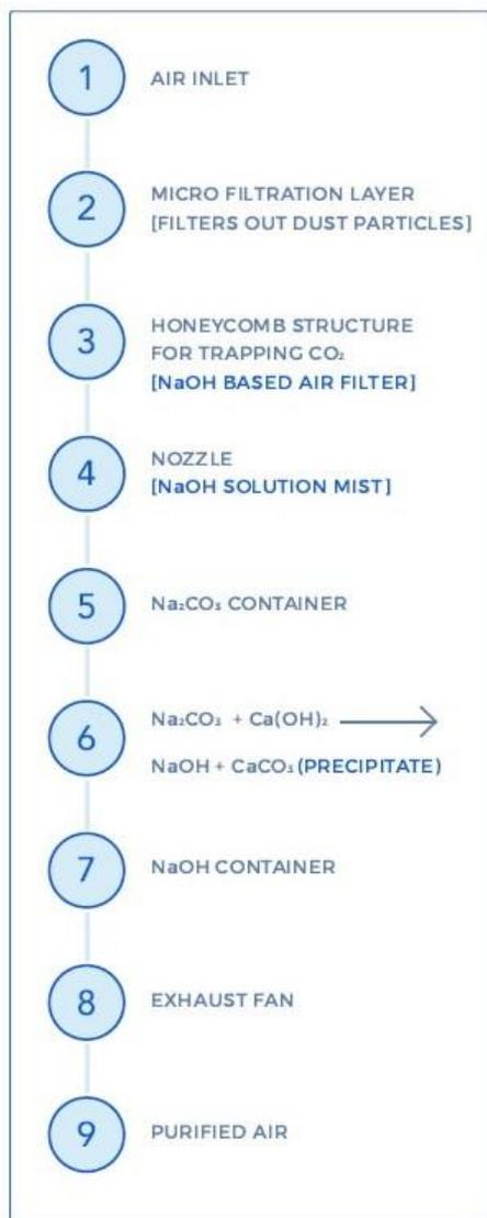
Figure 5: Working of prototype systematically
