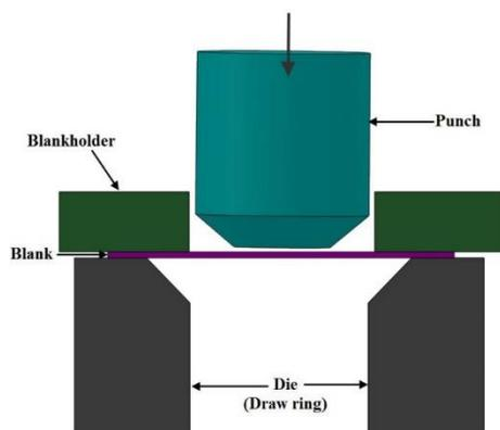
Fig-1: Diagram of Blanking Machine
