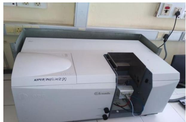
Figure 2 : Atomic Absorption Spectrophotometer
