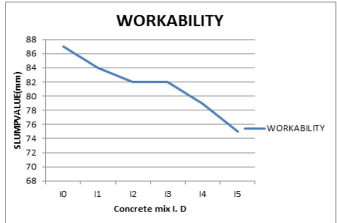
Figure Error! No text of specified style in document.: Workability Test for Different Mix
