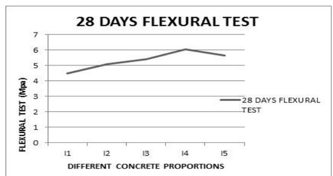
**Figure 10:** 28 Days Flexural Test for Different Concrete Mix
