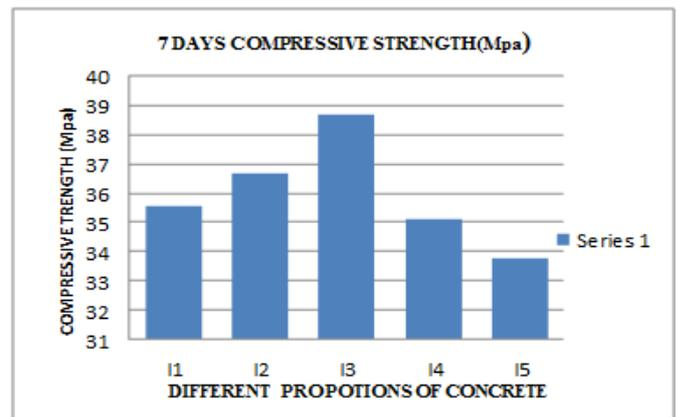
Figure 6: 7 Days Compressive Strength for Different Concrete Mix
