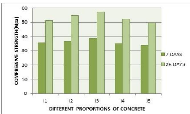
**Figure 8:** Comparison of 7 & 28 Days Compressive Strength of Different Concrete Mix
