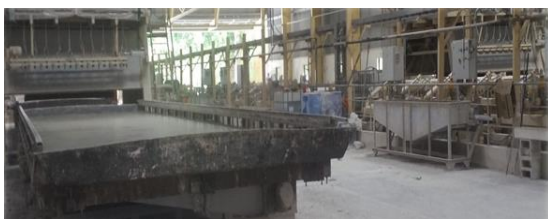
Fig- 4: Casting table in Wall Panel Plant
