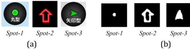
Fig. 1. Three types of laser pointers (a) color image (b) binary image[4]. Following that, a series of circuits are needed for the laser spot to communicate with the computer, which increases the cost largely.
