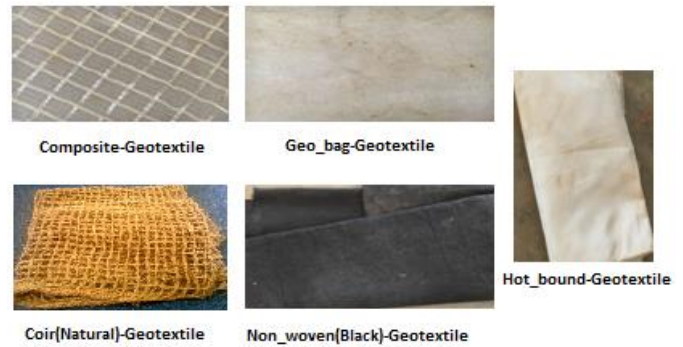
Fig -1: Reinforcement materials
