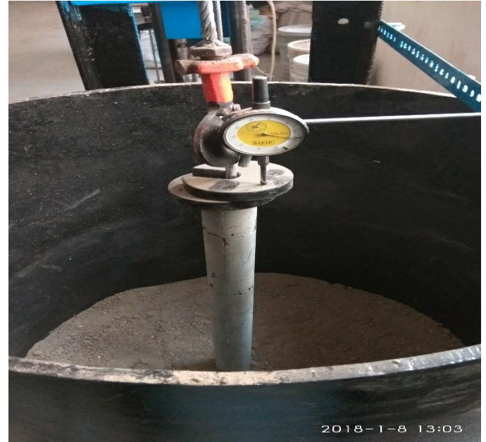
Fig3.2.1 showing the placement of dial gauge on single pile.
