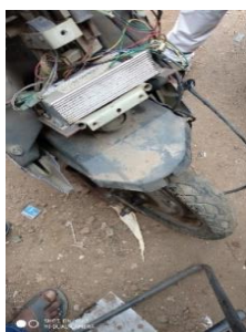
Fig 9-hub motor controller fixed in the front
