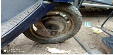
Fig 7-hub motor fixed in front wheel
