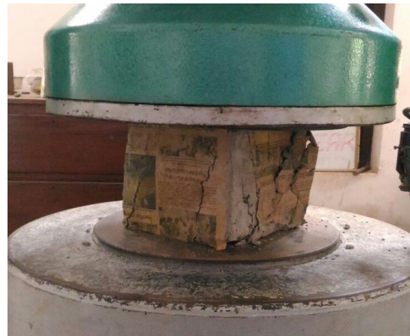
Fig-2: Testing of Geopolymer concrete cubes
