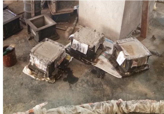
Fig-1: Casting of Geopolymer concrete cubes
