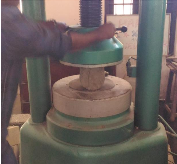
Fig-4: Splitting tensile strength test
