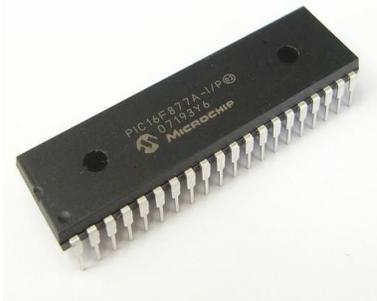
Fig. PIC Microcontroller 16F877A
