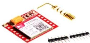
Fig. 3: GSM modem
