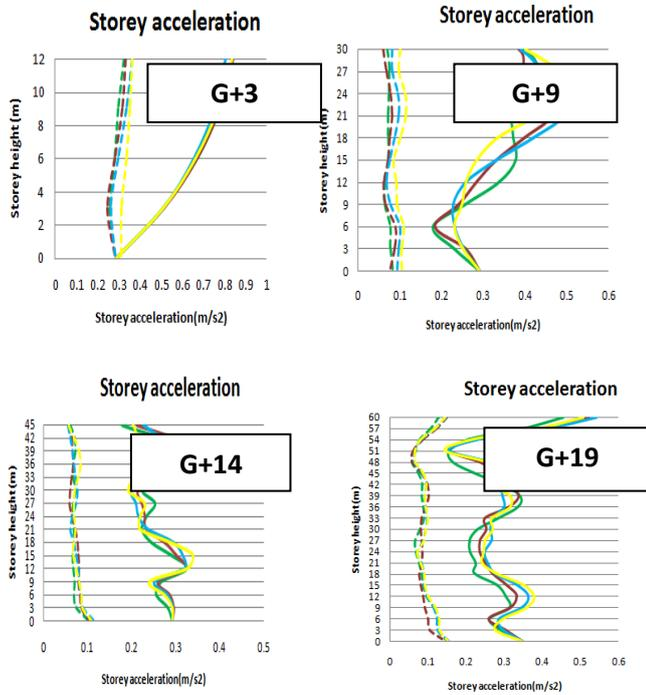
Fig 4 Maximum storey acceleration with storey height
