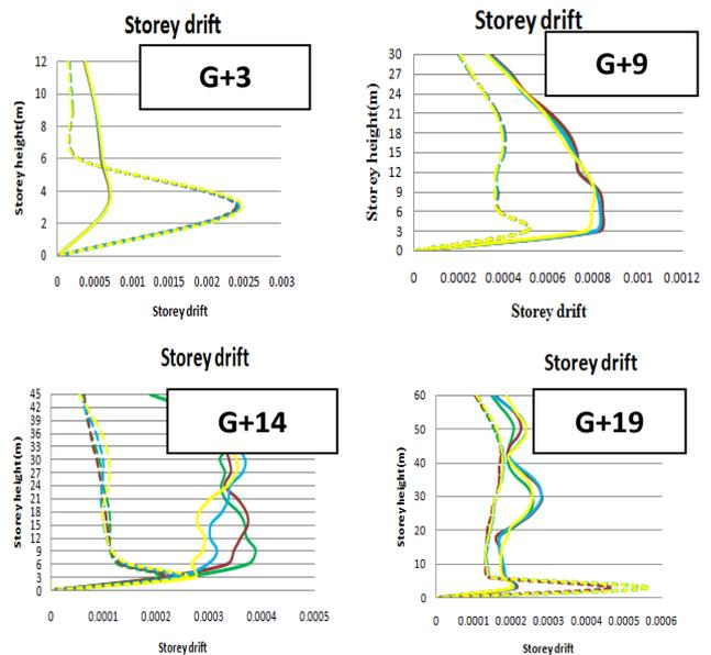
Fig 6 Maximum storey drift with storey height
