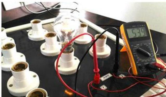
Fig-14: Photo of the load arrangement (Load voltage =53.9 V)
