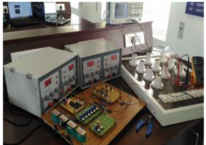
Fig-12: Hardware Setup for SPWM based nine Level Inverter
