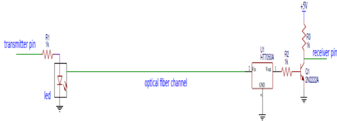
Fig:2.circuit connection for optical communication system
