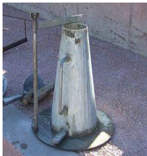
Fig-2: slump of concrete
