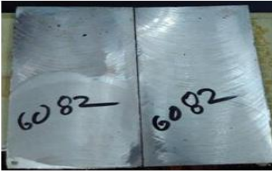
Fig 2. Work piece before friction stir welding
