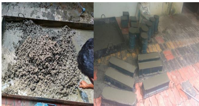
Fig-8: Stages of preparation of specimen (a) Mixing (b) Casting
