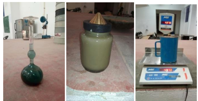
Fig-2: Specific gravity test on a) cement b) fine aggregate c) coarse aggregate
