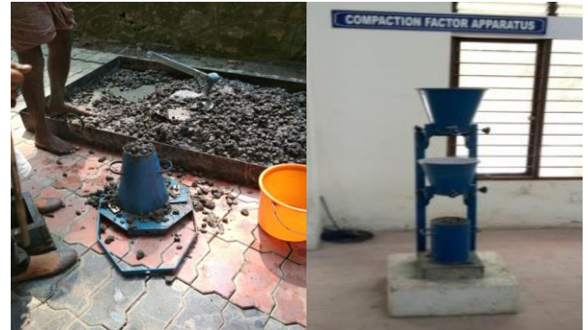
Fig-9: Workability test (a) Slump cone test (b) Compaction factor test
