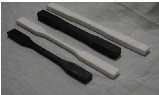
Fig-5. Specimen of ASTM D638
