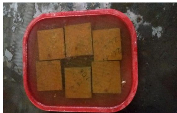
Fig. 2 Test setup of acid attack
