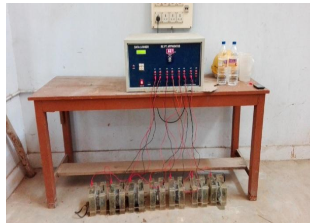
Fig. 4 Test setup of Rapid chloride penetration
