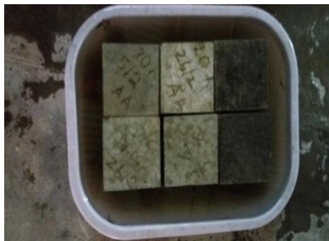
Fig.3 Test setup of sulphate attack
