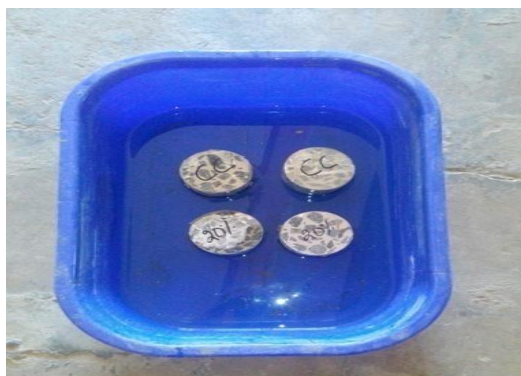
Fig. 5 Test setup of Sorptivity Test
