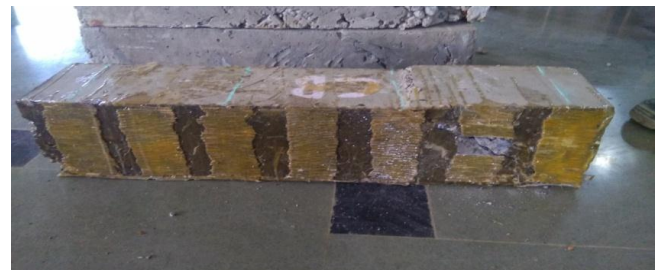
Fig -14: CB9 after testing
