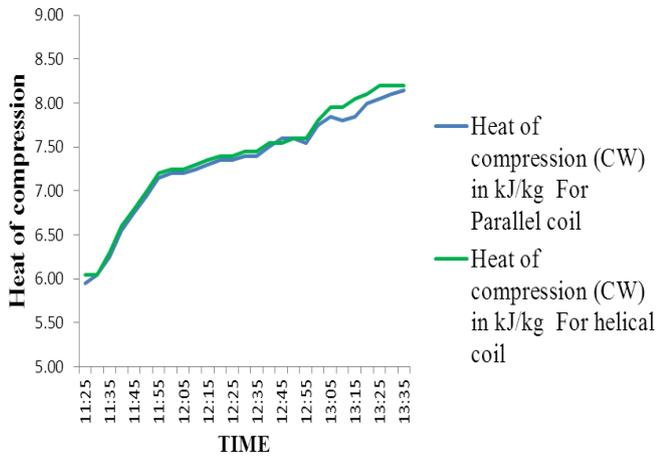
Chart -3: Compressor work For parallel Vs Helical coil condenser
