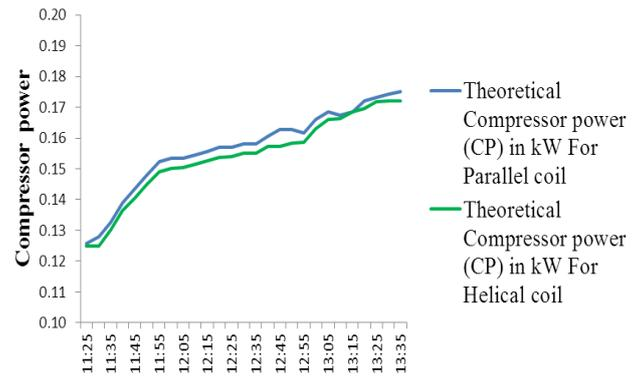
Chart -5: Theoretical power For parallel Vs Helical coil condenser
