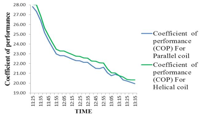
Chart -6: COP For parallel Vs Helical coil condenser
