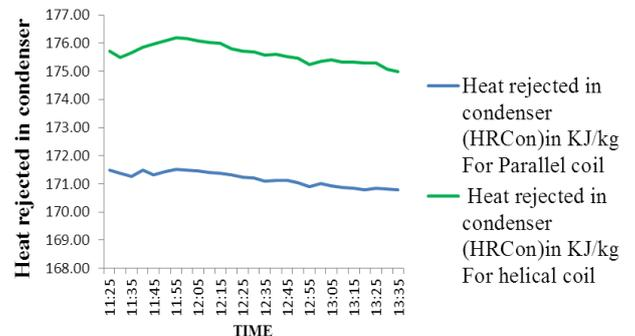
Chart -7: Heat rejected in condenser For parallel Vs Helical coil condenser
