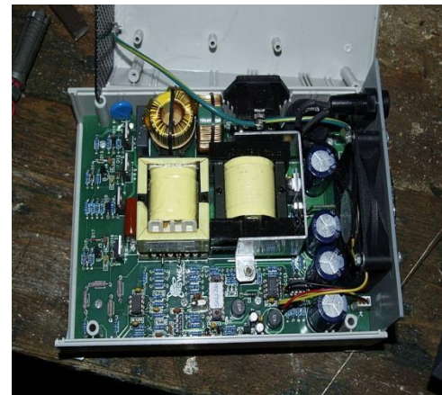
Fig.1 Grid Tied Inverter
