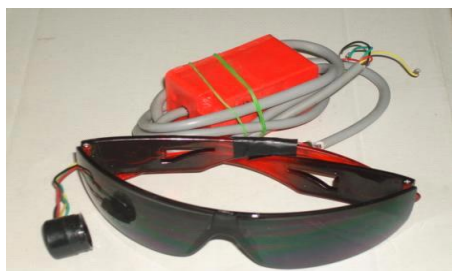
Figure4: Head gear using IR sensor
