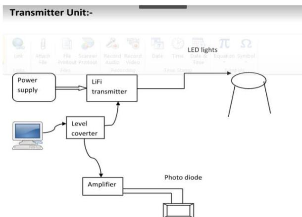
Here the user sends the required data to be fetched to the server by means of lifi transmitter through level converter. The data is then transmitted through an LED lights to the server and the photo diode which is the receiver used to receive the data required by the user by means level converter.
