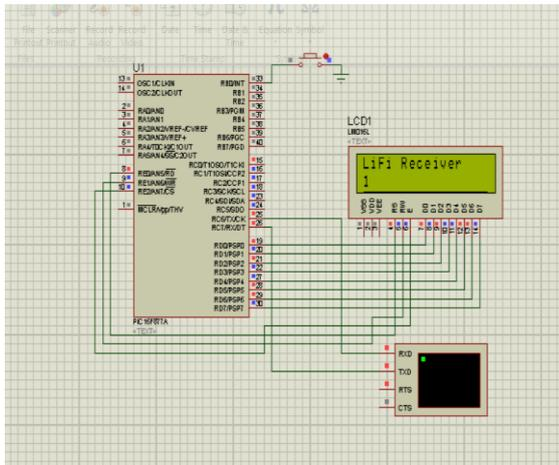
The data which is transmitted from the user through LIFI transmitter is received to the source by means of LIFI receiver. The required data is fetched from the source and again it is sent to the user by the same means of transmitting and receiving process. The simulation for data receiver is shown above.
