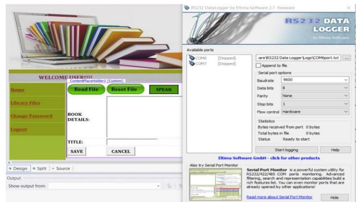
In this library system, a RS 232 Data Logger app is installed at the library side PC to correctly read and fetch the data required by the user in the proper manner. In the same way the data is transmitted from library system to the user by means of LIFI transmitter and LIFI receiver.
