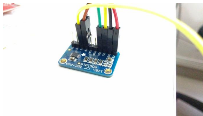
Fig - 8: ADS1015 connected with sensors
