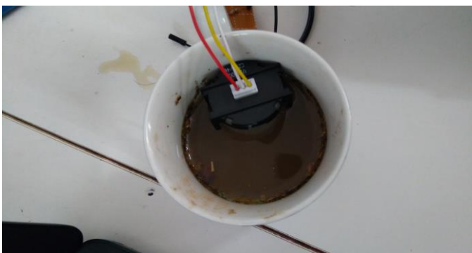
Fig - 12: Collecting turbidity value from dirty water
