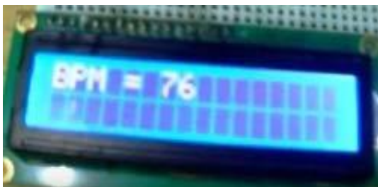
Fig. 6 LCD showing heart beat in BPM
