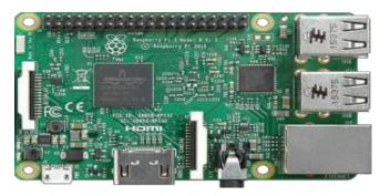
Fig-1.1 RaspberryPi3ModelB board
