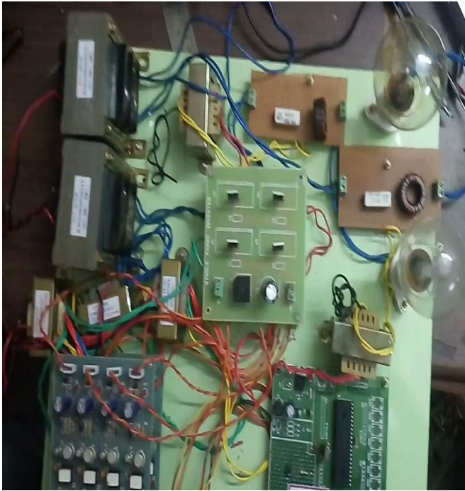
Fig 4.1 : hardware of IDVR
