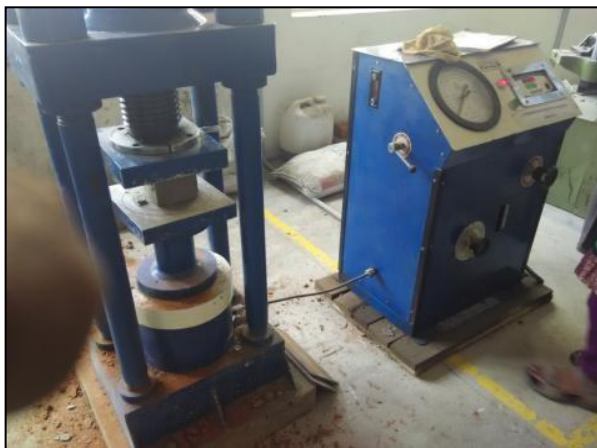
Fig.4 Compression test setup
