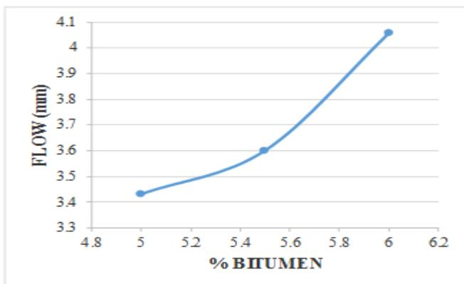
Chart -3: % Bitumen vs Flow graph
