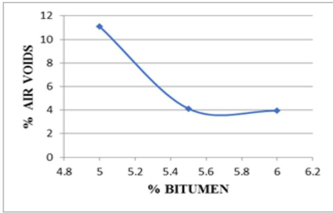
Chart -1: % Bitumen vs % air void graph
