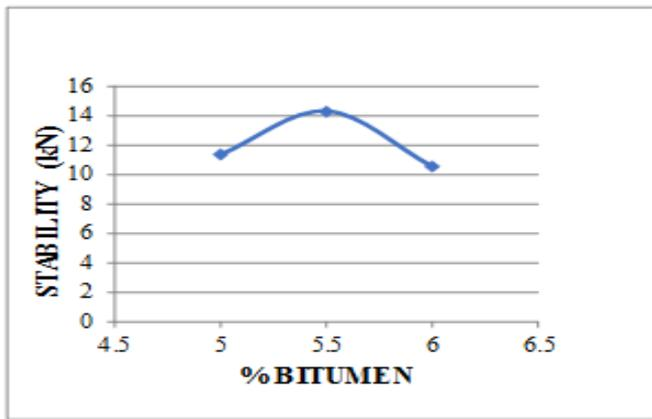
Chart -2: % Bitumen vs Marshall Stability graph
