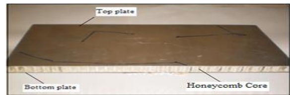
Fig - 1 Honeycomb Core
