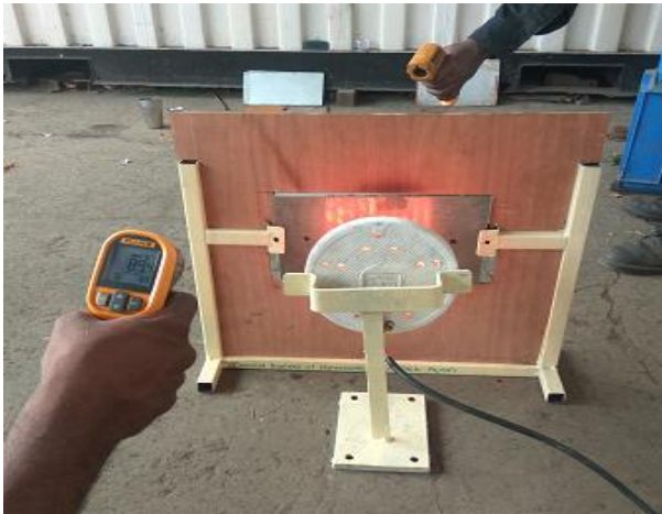
Fig-11 Actual Experimental Set Up for 15 mm Composite Hexagonal Honeycomb Panel
