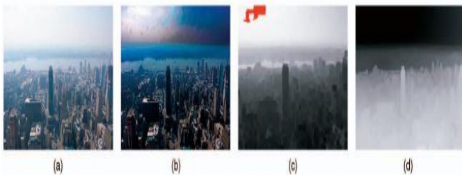
Fig-6: Haze imaging model failure case; (a) foggy image; (b) Result of the study; (c) Dark channel; (d) Estimated transmission map.
