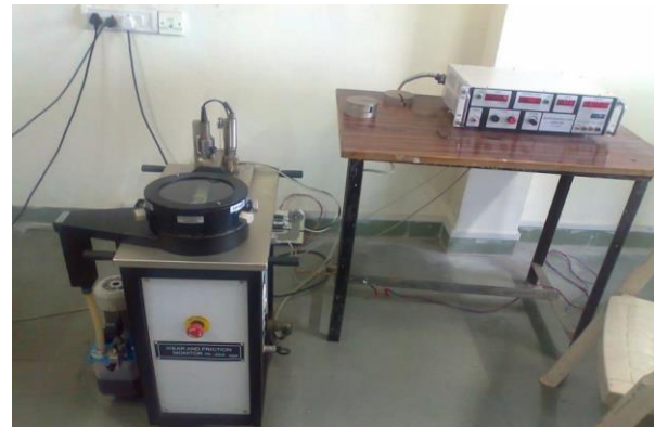
Fig. 3.2 Photograph of experimental set up (Tribometer TR20LE-PHM-400).
