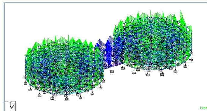
**Fig -4:** Live load diagram
