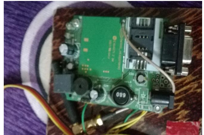
Fig.2: GSM Modem SIM 300
