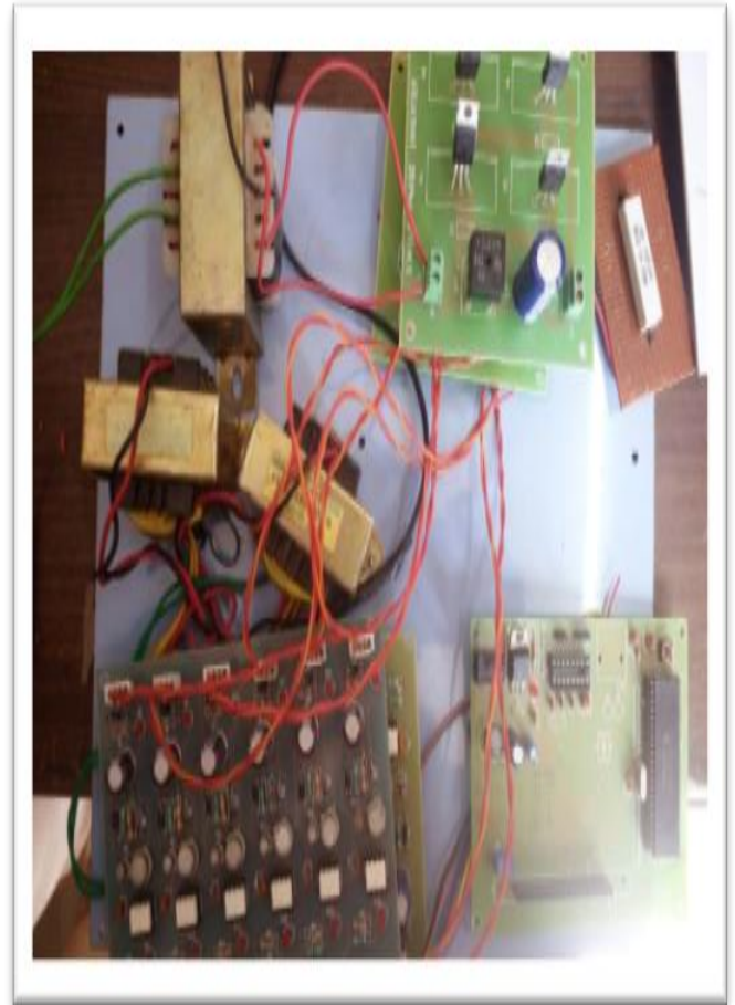
Fig-6 Hardware photo of 15 level multilevel inverter.
