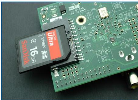
Fig.5. SD card installation
