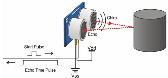
**Fig.2.5. Ultrasonic sensor**
