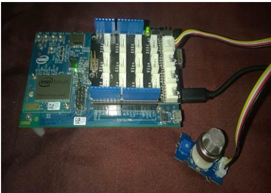
Fig 4.3 Intel Galileo connected to gas Sensor
