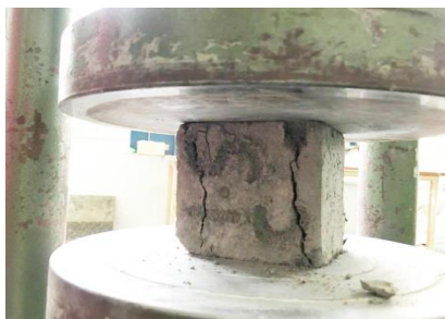
Fig -2: Compressive strength test of mortar
