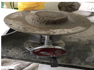
Fig -1: Flow table test of mortar
